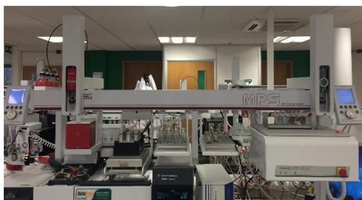
Figure 2. Showing Automated Vortex (mVORX) and Centrifugation (CF-200) using a Dual Head XT MultiPurpose Sampler on a GC/MS 5975
