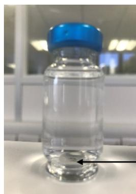
Figure 3 – High recovery vial with low volume of the dichloromethane present at the bottom of the vial
