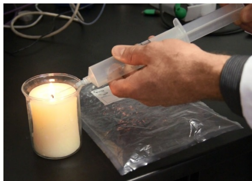
Figure 3: Sampling of combustion products from wax candle flame.
