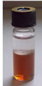
Sample vial after hair digestion, extraction and centrifugation. A clear phase separation between the upper organic extract phase and lower aqueous phase (dissolved hair) is achieved.
