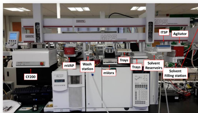
Figure 2: GERSTEL Dual Rail MPS with Agilent GC-MS for fully automated determination of opiates in blood
