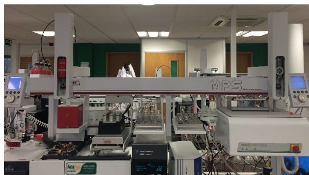
Figure 2. Automated Vortex (mVortex) and Centrifugation (CF-200) using a GERSTEL Dual Head xt MultiPurpose Sampler on an Agilent Technologies 5977B High Efficiency Source, GC/MSD and 7890B GC
