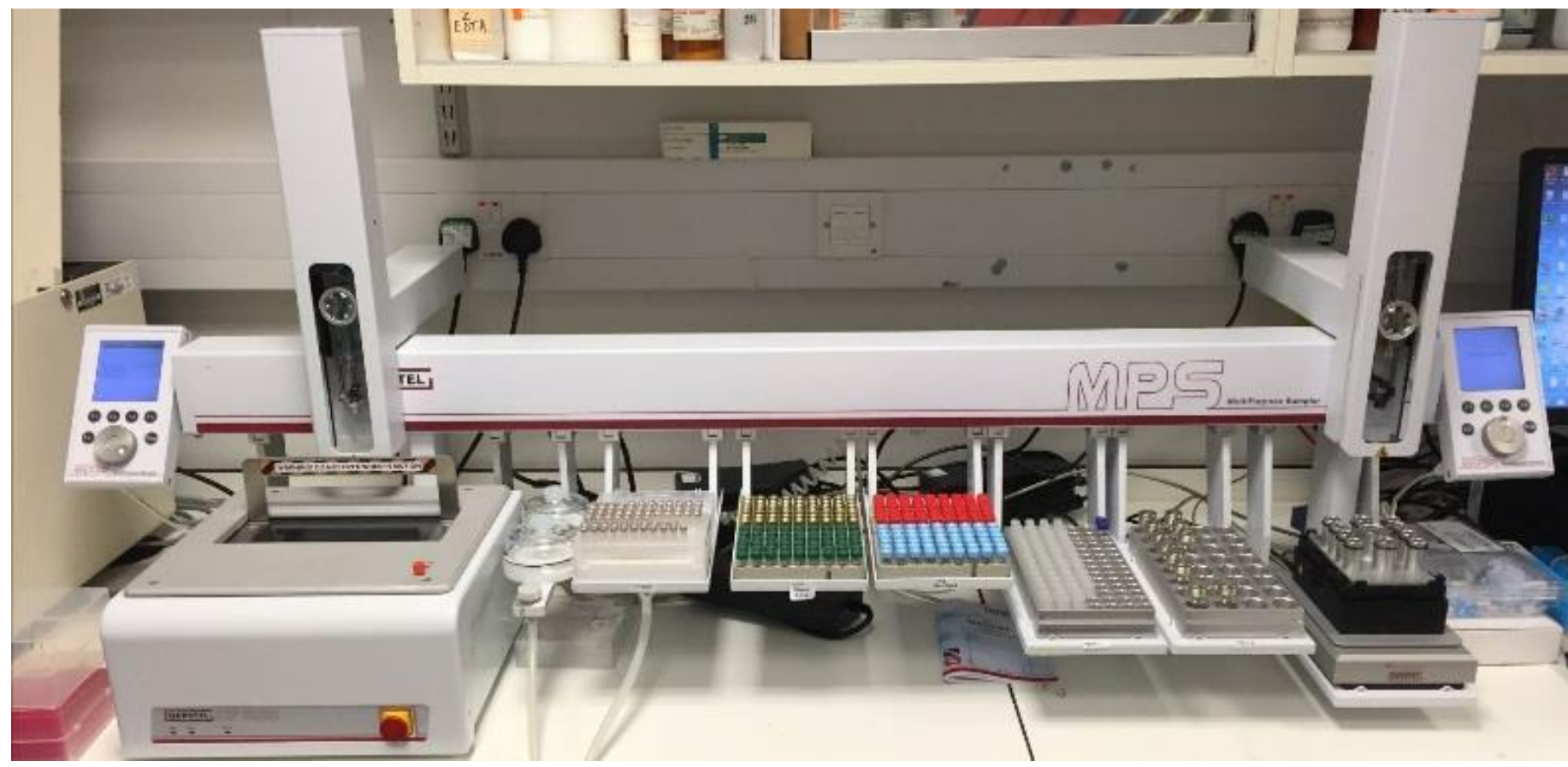
Figure 1 – Anatune Amino Acid Solution comprising GERSTEL Dual Head Multi Purpose Sampler with GERSTEL Multi-position Vortexer (mVORX), Anatune Robotic Centrifuge (CF-200) and SmartSPE™ (ITSP Solutions Inc) options
