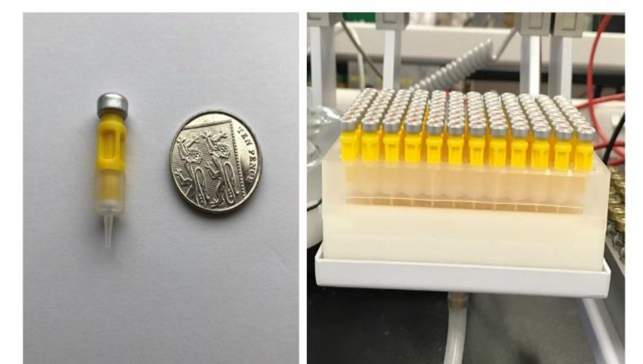
Figure 2 – SmartSPE™ Instrument Top Sample Preparation micro-scale (μSPE) solid phase extraction cartridge and 96-well format tray
