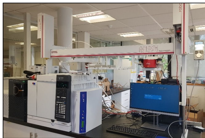
Figure 1: GERSTEL Dual Head Robotic MPS on top of Agilent GC 7890B coupled to 7250 Q-TOF MS
