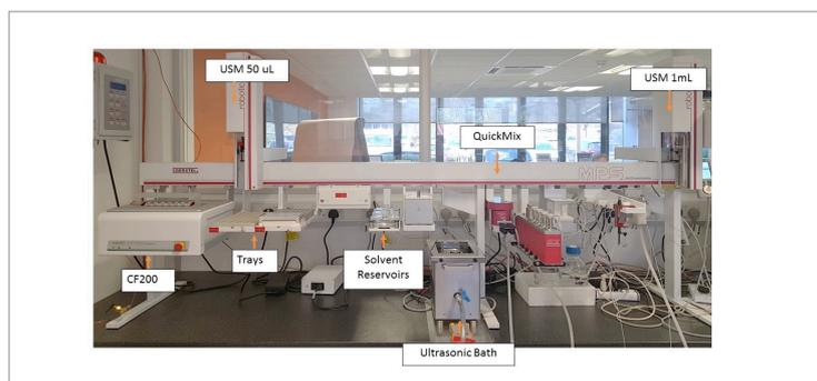
**Figure 2:** Automated sample preparation system for extraction of steroids from Mitra® microsampling device
