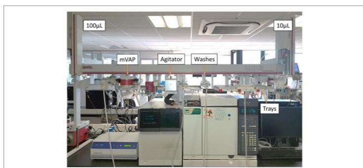
**Figure 3:** Online automated solution for the derivatisation and GC-MS-MS analysis of steroids from Mitra® microsampling device
